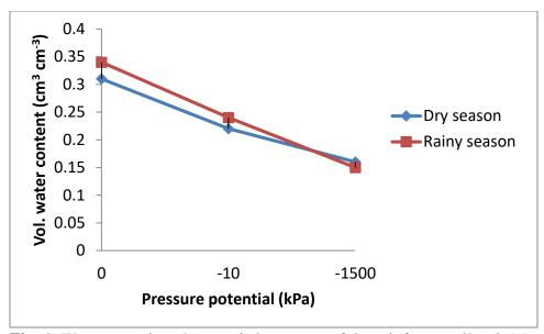
**Fig. 1.** Water retention characteristics curves of the rainforest soil at 0-15 cm topsoil during the dry and rainy seasons
