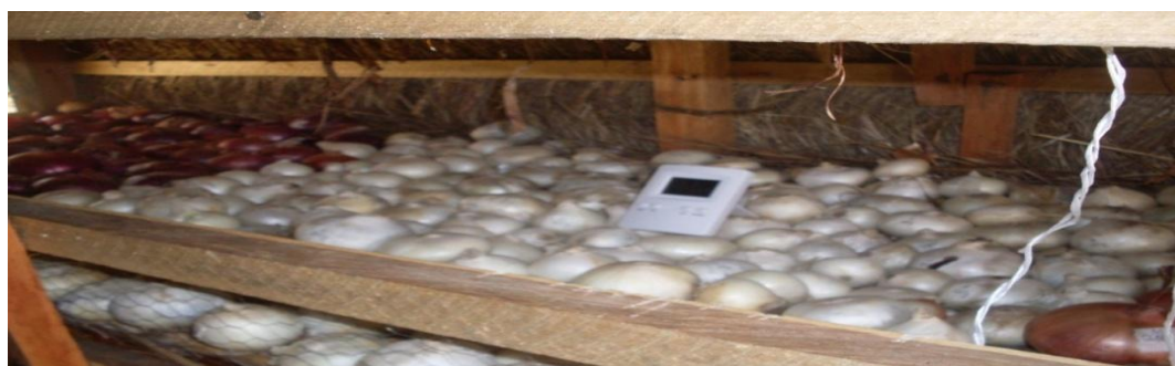
Plate 1: Digital Thermo-hygrometer for measuring temperature and relative humidity in the storage structure
